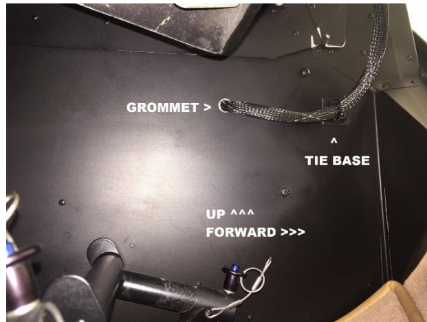
Figure 10: Grommet and Cable Tie Base Installation
