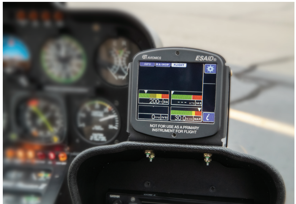
Figure 1: Surface mounted ESAID®.
